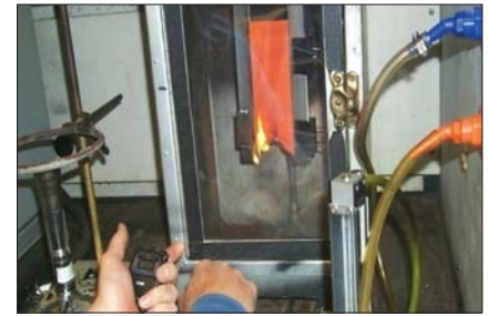
Fig. 1: The ASTM D6413 vertical flame test.
